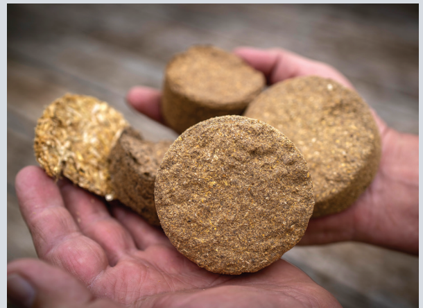
The company already produces bio-fuel briquettes from production wastes for use in industrial boilers as an alternative to coal.
