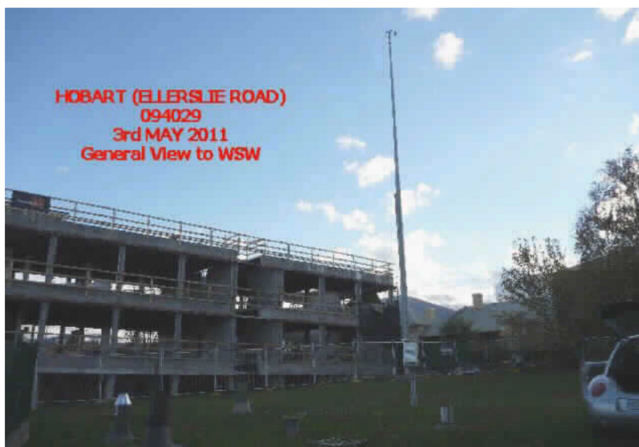
Figure 39. Battery Point (Hobart) Ellerslie Rd. meteorological observing site with 20 metre anemometer mast (view to WSW illustrating the redevelopment of a 3-storey structure). Image supplied by the Bureau of Meteorology, Hobart office.
