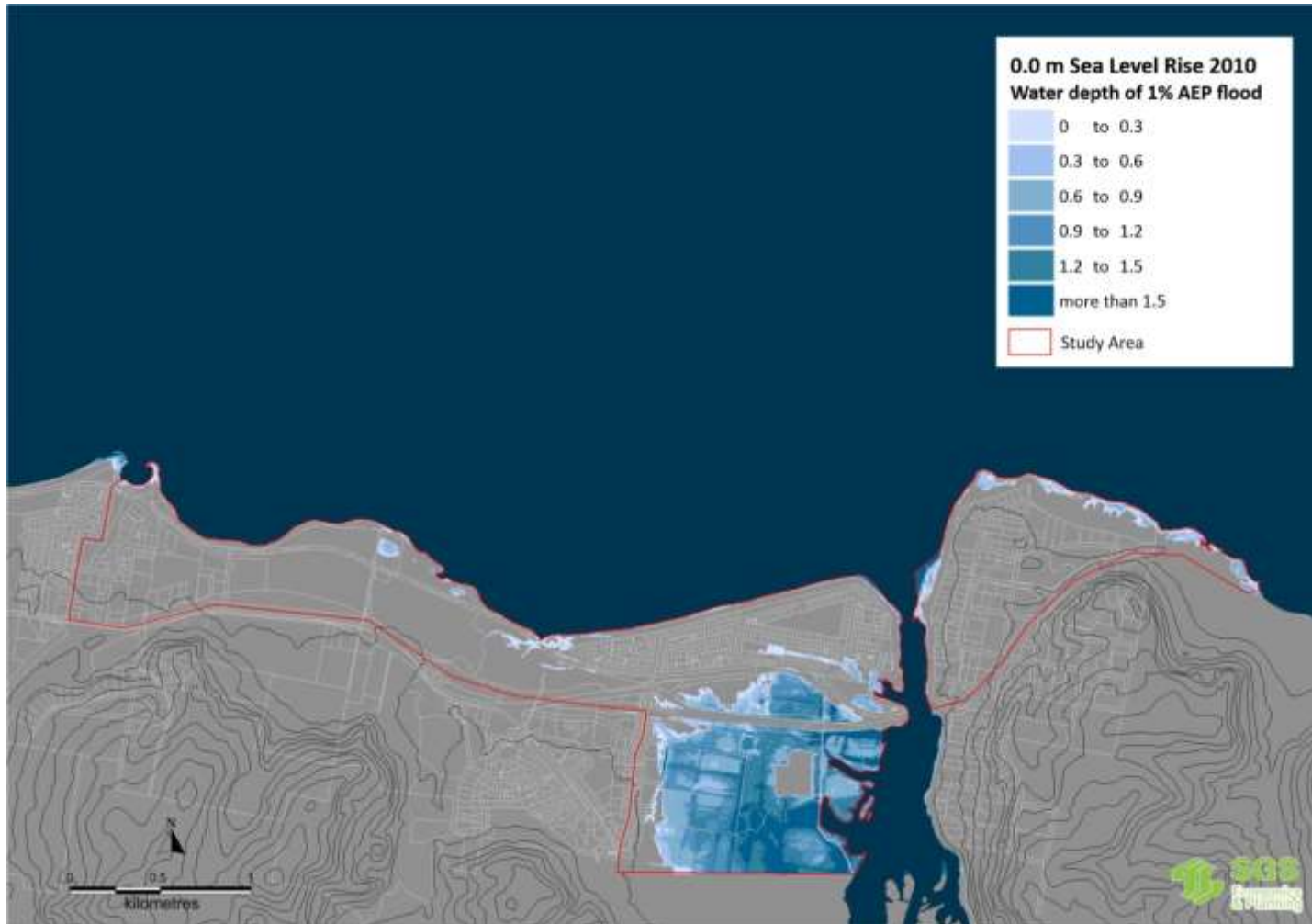
FIGURE 2 LIKELY INUNDATION DEPTHS AT TURNERS BEACH AND LEITH FOR AN EXTREME STORM EVENT (1% AEP), PRESENT DAY
