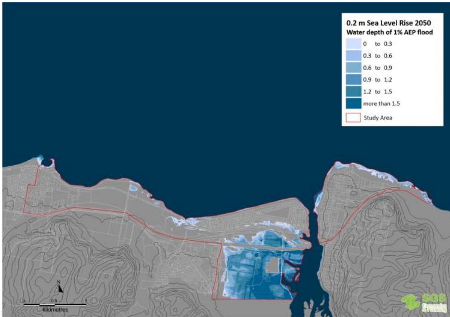
FIGURE 4 FIGURE 4 LIKELY INUNDATION DEPTHS AT TURNERS BEACH AND LEITH FOR AN EXTREME STORM EVENT (1% AEP), 0.2 M SEA LEVEL RISE
